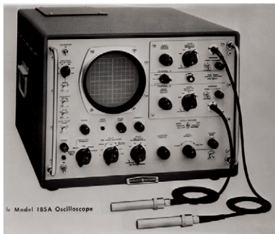
Many engineers still like analog oscilloscopes, such as the HP Model 185, built in the 1960s. Courtesy of Agilent Technologies.
